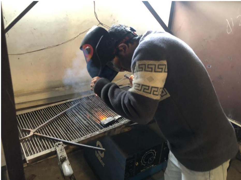
Fig A16. Welding of Test Specimen
