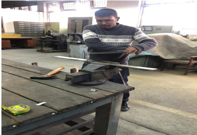
Fig A12. Bolt Pre-Tension With Calibrated Torque Wrench
