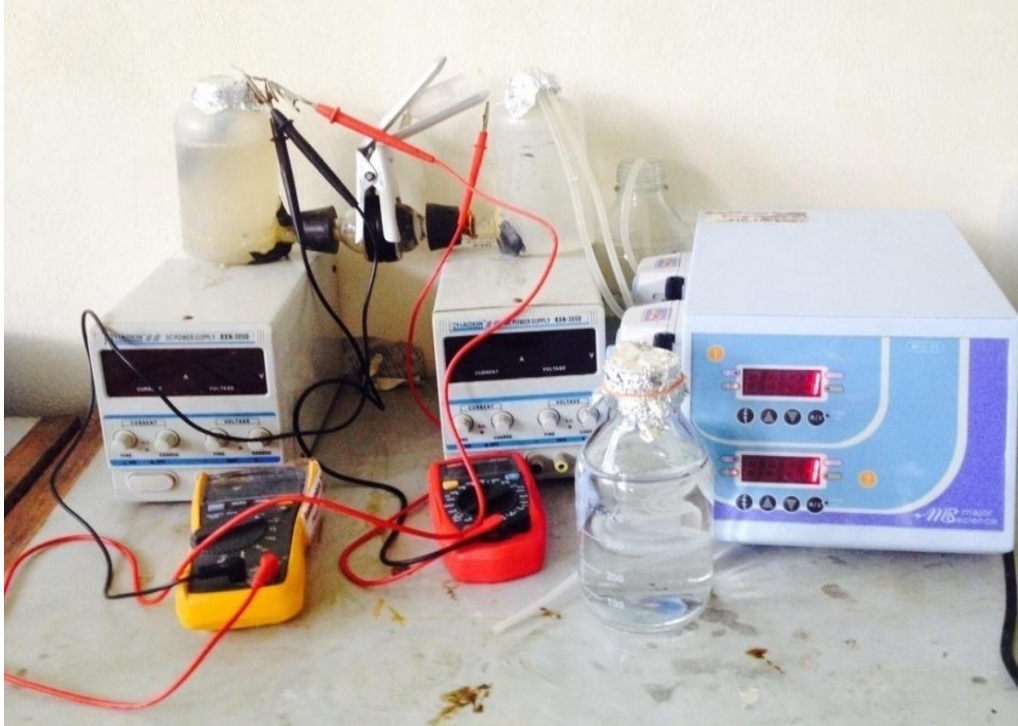
Figure 3.1: Microbial Fuel Cell with the addition of Hydrogen Peroxide using a peristaltic pump.
