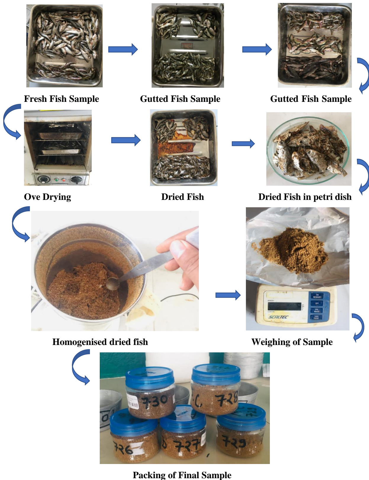
Figure 3: Process of sample preparation of small indigenous fish species for proximate analysis.
