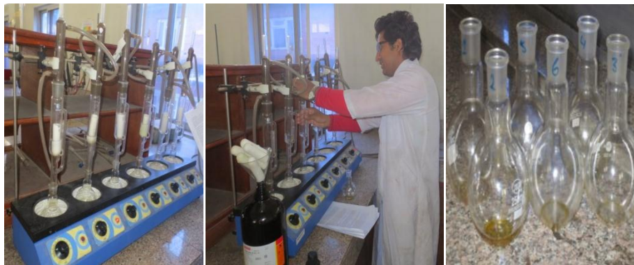
6: Fat estimation by using Soxlet apparatus
