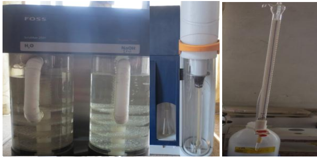
5: Protein determination(Digestion, Distillation, Titration)
