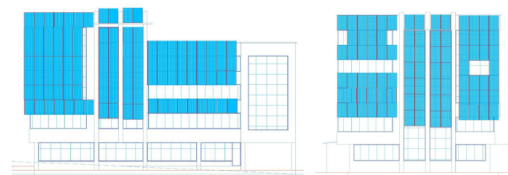
Figure 5: Placement of calculated BIPV in the east and south facade of case building
