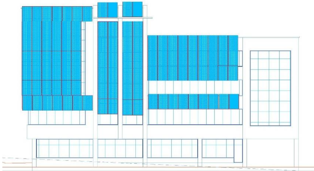
Figure 5-19: East elevation with solar panels
