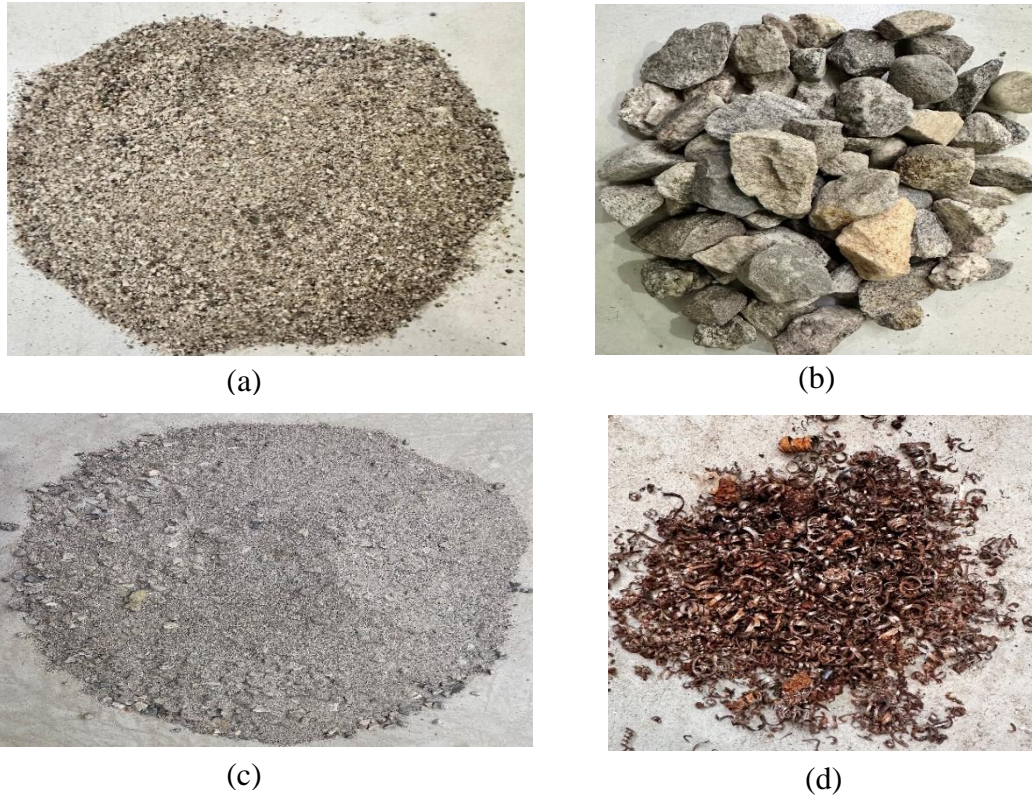
Figure 3.5: TES material sample, (a) Silica sand, (b) Aggregates, (c) sand aggregate uniform mixture, and (d) Scrap cast iron metal chips.
