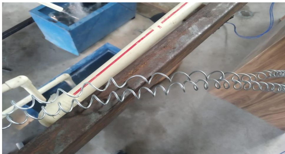
Figure 3.12: Helical Coil Turbulators
