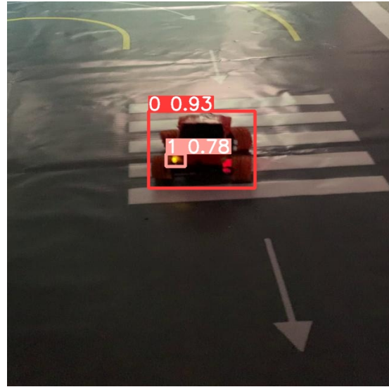
(d) Detection of car and silight with 0.93 and 0.78 confidence score respectively
