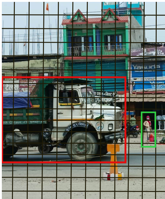
Figure 2.6: Bounding Box Creation in Grid
