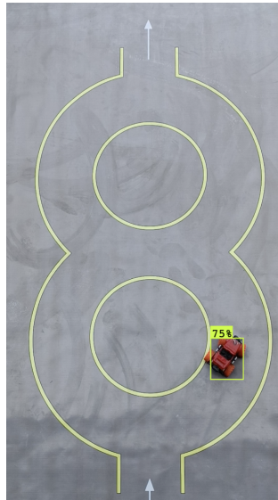
Figure 5.7: Bounding Box prediction of the vehicle in 8-test
