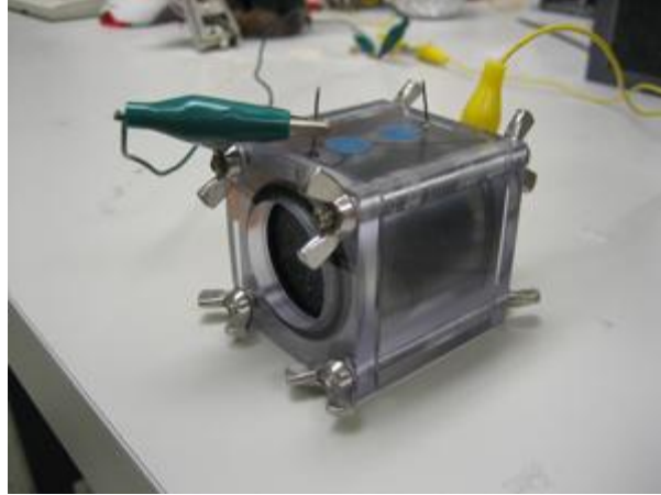
Fig2.2: A single-chamber MFC (courtesy of Penn State)
