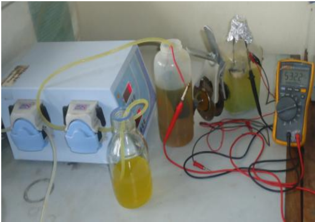
Fig3.2 Microbial fuel cell with the drop wise addition of Potassium ferricyanide and Phosphate buffer using the peristaltic pump.
