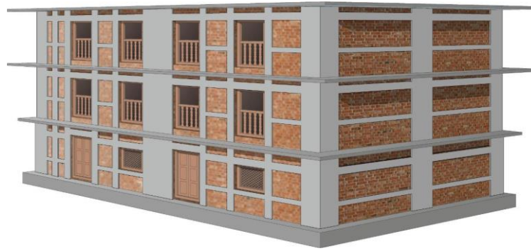
Figure 3.25 Retrofitting with concrete and rebar Jacketing with splint-bandage and GI wire mesh (Brick masonry)
