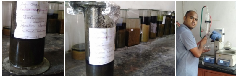
Cold percolation in methanol extract crude methanol extract by rota vapor
