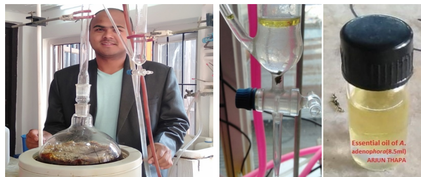
Hydrodistillation process by Clevenger apparatus and essential oil of A. adenophora
