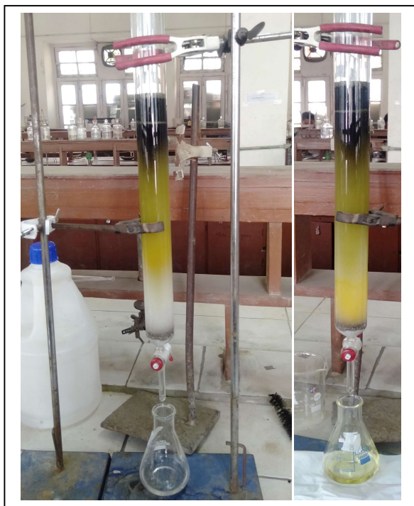
Figure 47: Column chromatography of A. adenophora leaves methanol extract.
