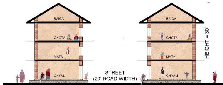
Figure 39: Section of Asan-Bhotahity Road(Past)
