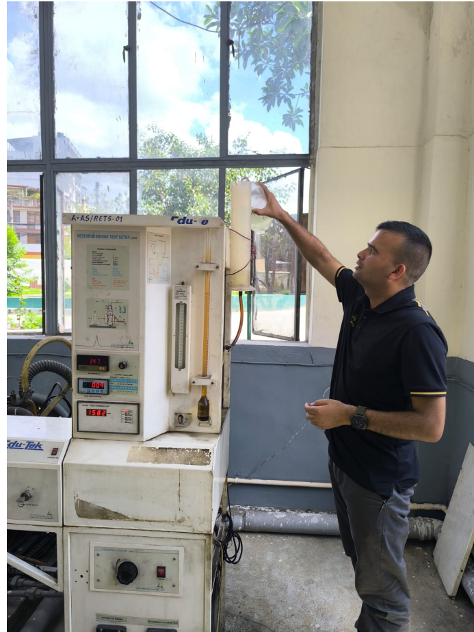
Figure 5.6: Refueling test engine with biofuel sample
