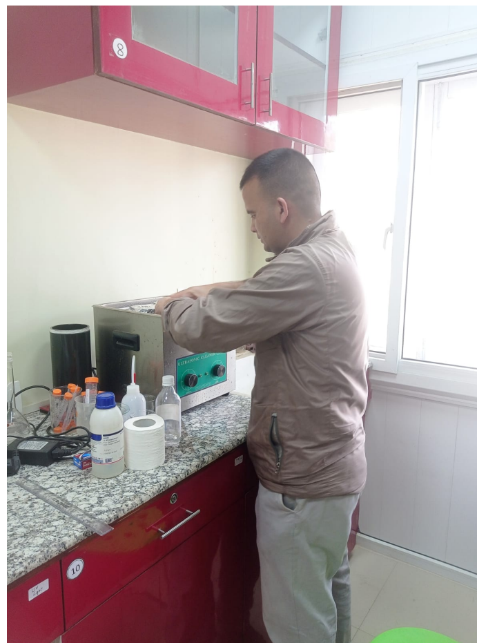
Figure 5.3: Sonication of nanoparticles with fuel blends
