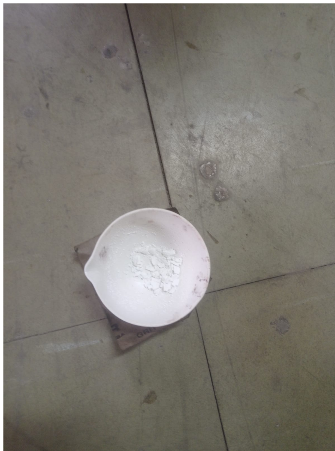
Figure 5.1: Synthesized Al 2 O 3 nanoparticles in laboratory
