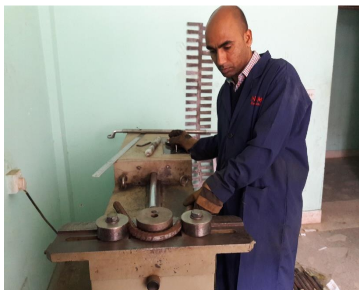
Figure 3.5 Bend and re-bend test machine at NBSM
