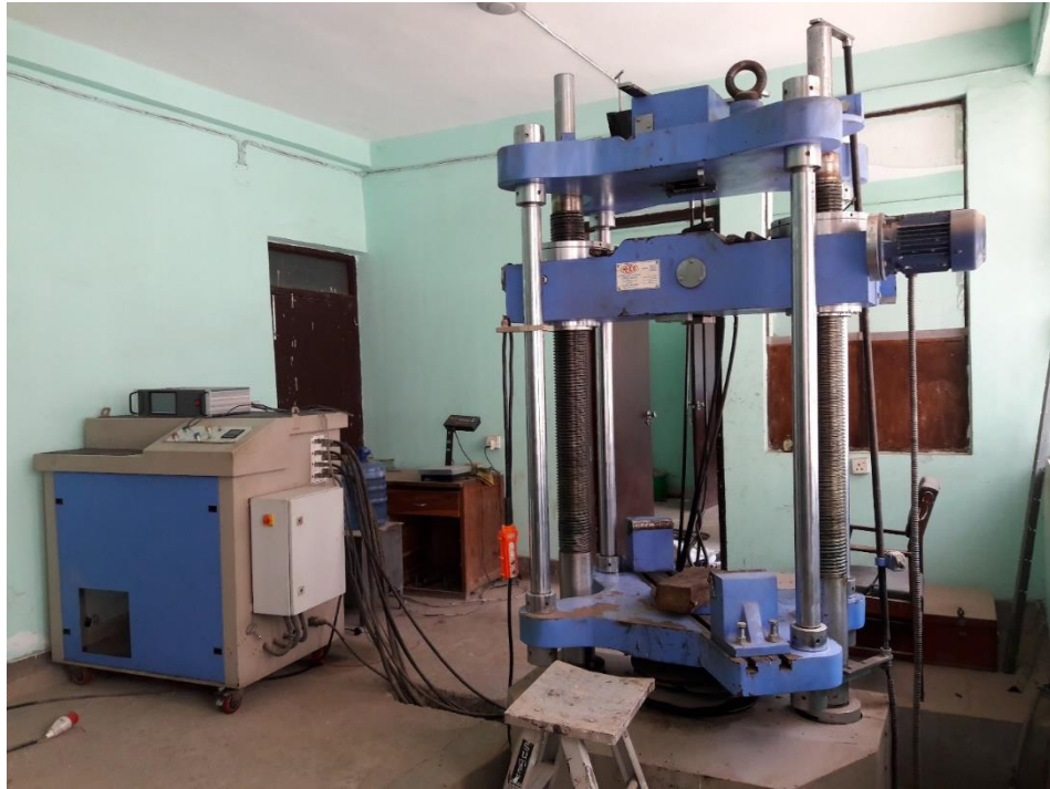
Figure 3.4 Heico UTM machine 1000 kN at NBSM mechanical testing laboratory
