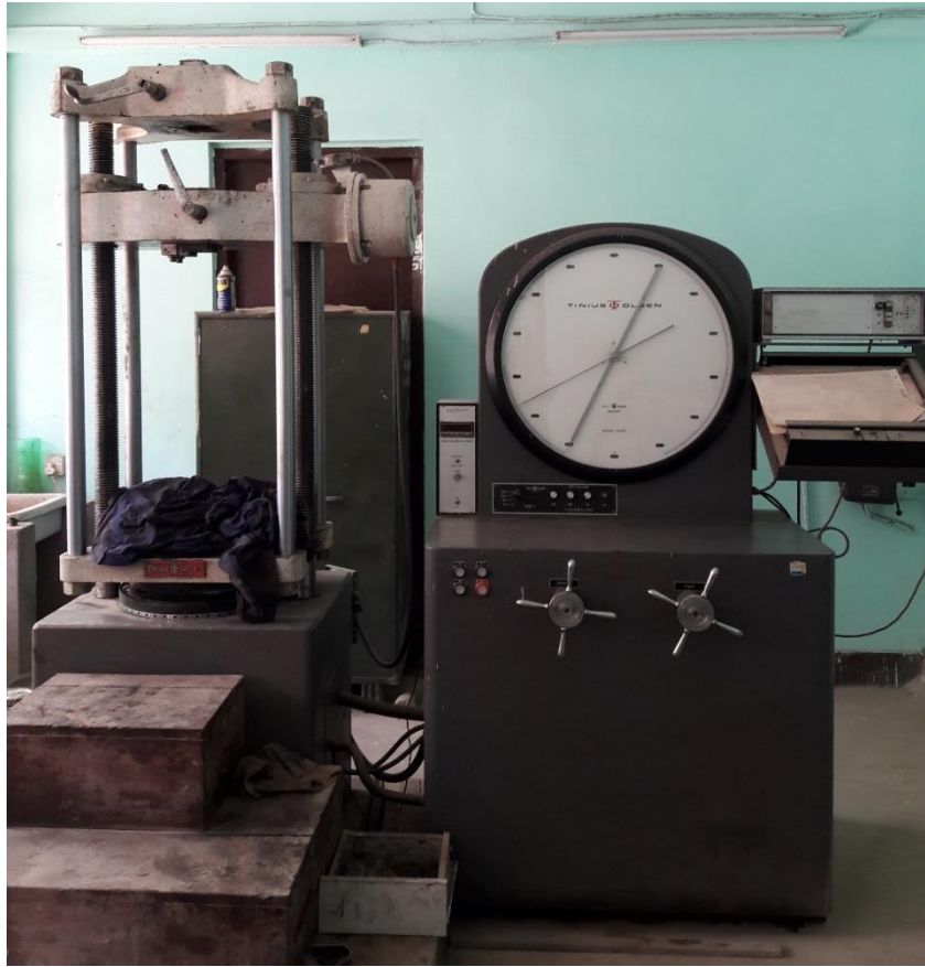
Figure 3.3 Tinus Olsen UTM machine 600 kN NBSM mechanical testing laboratory
