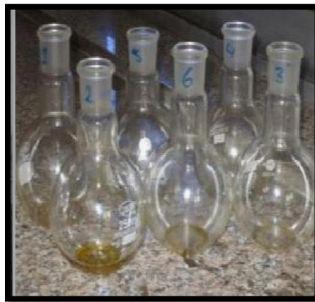
Photo 3 Fat estimation using Soxhlet apparatus
