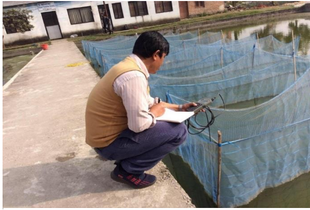
Photo 7: Measuring of water parameters of the ponds by using Multiparameter meter
