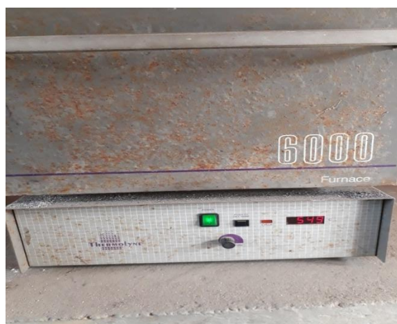
Fig: Muffle furnace at 500°C
