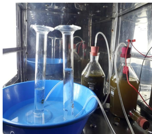
Fig: 1L setup of MEC and control
