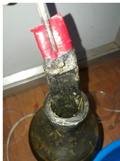
Fig: C-felt electrode after 15 days of setup
