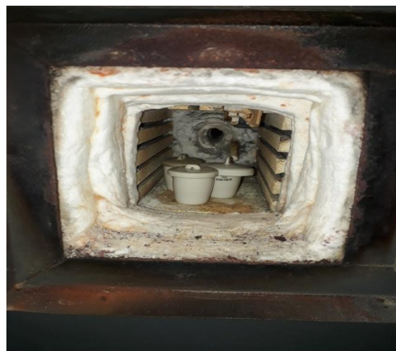
Fig: Crucible mug inside muffle furnace
