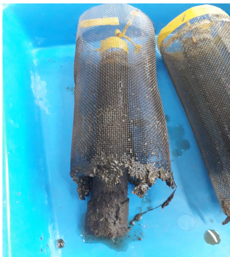
Fig: Corroded steel electrode after 15 days of setup
