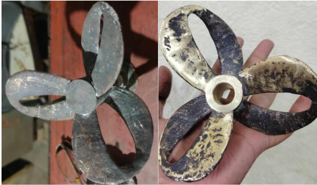
Figure 26:- Turbine Obtained After the Casting Process
