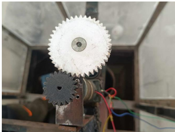
Figure 28 Gear system connecting shaft to dynamo
