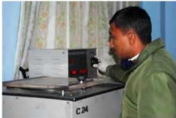
Photo 4A. Using REMNI® C24 cooling centrifuge Photo 4B. Template DNA in micro-centrifuge tubes
