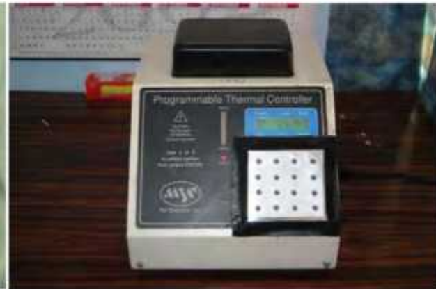
Photo 4C, D. Placing PCR Beads (left) and running program (right) in Programmable Thermal Controller, MJ Research Inc.
