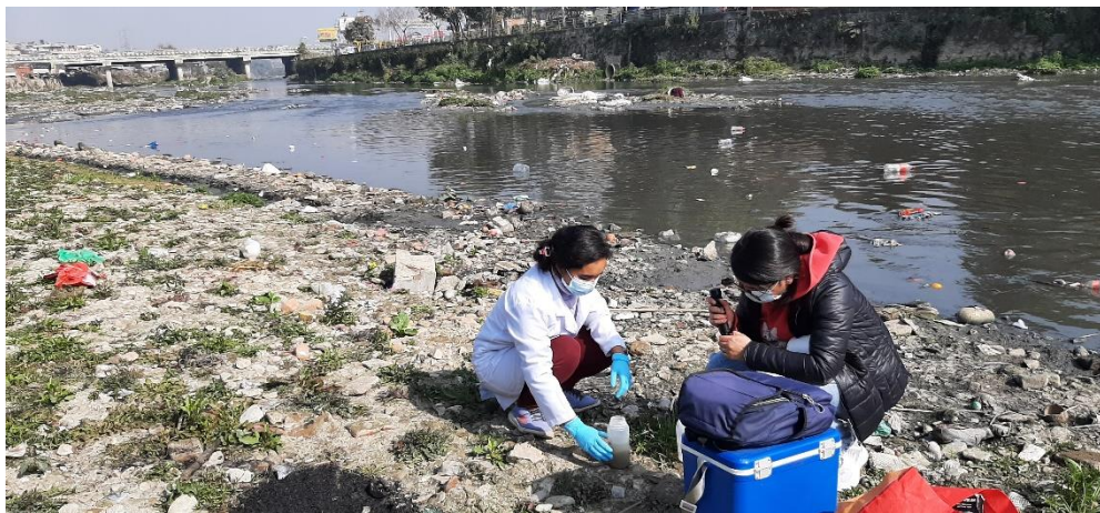
Photo 2: On-site Temperature and pH determination of the sample using a portable machine at the sampling site
