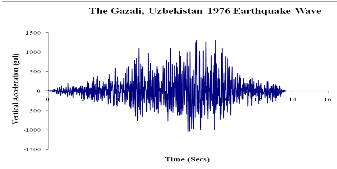
Fig4.15: Input Earthquake Wave (Vertical Acceleration)
