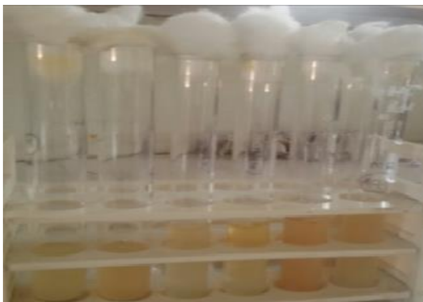
Figure 4.6 Methyl Red test of isolated Geobacter sps; no color changed of media
