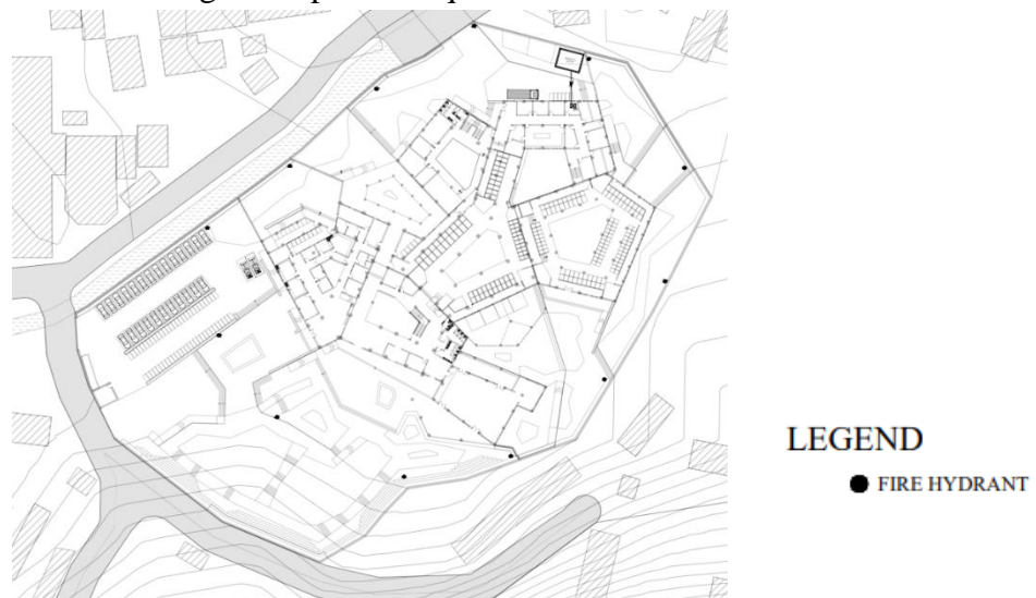
Figure 197: Fire Hydrant Layout
