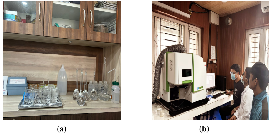
Figure 3.7: (a) Sample prepared for ICP-OES. (b) Sample testing in ICP-OES.
