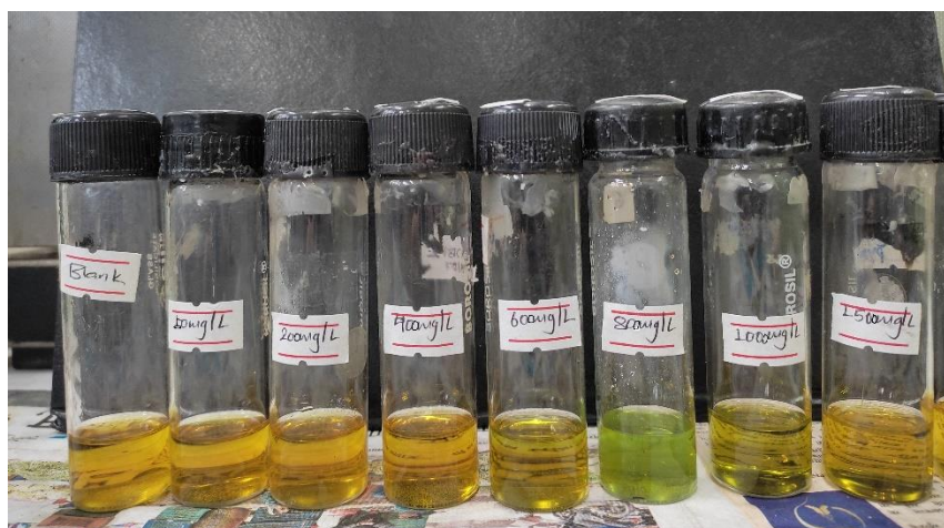
Figure 5: color observed of digested standard during COD determination
