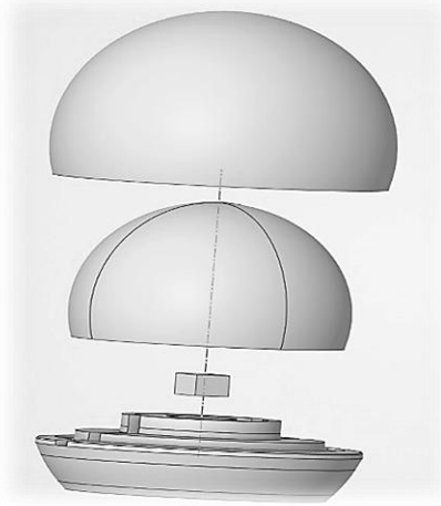
Figure 4.18 CAD Model of Headform Components
