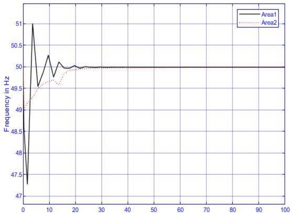
Figure 24: Frequency response of system with ANFIS controller
