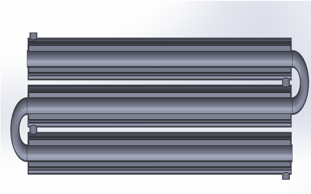
Figure 4.26: Side view of the concentric PCM heat storage setup
