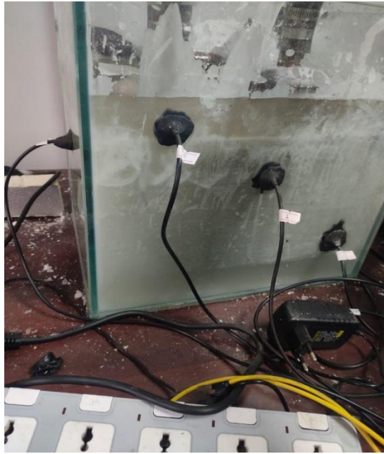
Figure 4.56: Temperature sensors attached to the glass surface
