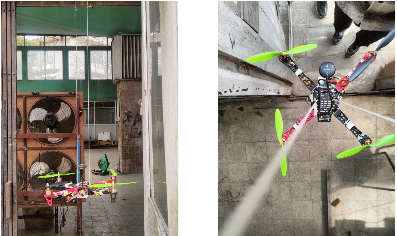
Figure A.1: Bifilar Pendulum Experiment for MOI determination
