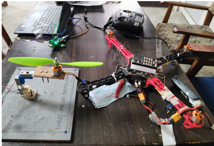
(a) Maximum Thrust Calculation using Load cell
