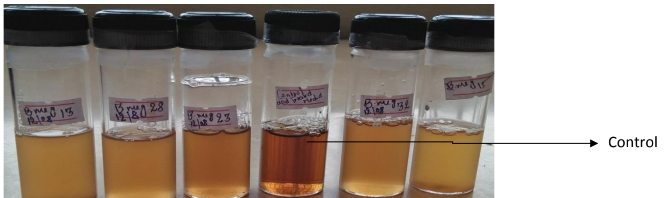
Figure 34: Growth of Bacillus megaterium in acid treated lignocellulosic biomass.
