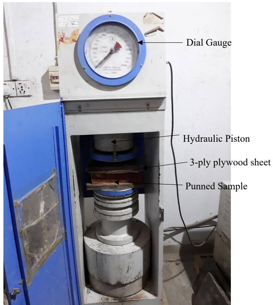
Figure 12 Compressive strength testing of brick
