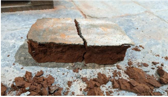
Figure 30 Failure of sample along center
