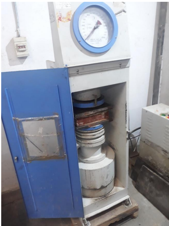
Figure 27 Compressive testing of brick sample
