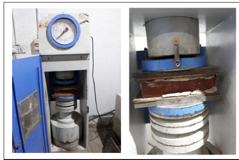
Figure 4: Compressive strength testing
