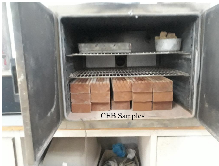
Figure 7 Air oven drying of bricks at 250°F
