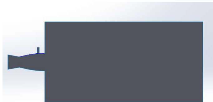
Figure 6.1: Geometry of nozzle along secondary inlet and flow domain behind the nozzle
