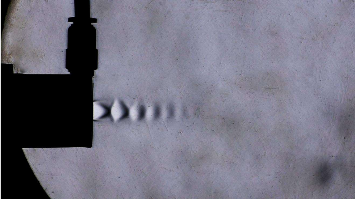
Figure B1: Schlieren images for jet deflection corresponding to NPR = 11 , SPR = 0.7 and when the secondary inlet located at (a) 25 %, (b) 50 % and (c) 75 % of the divergent section length
