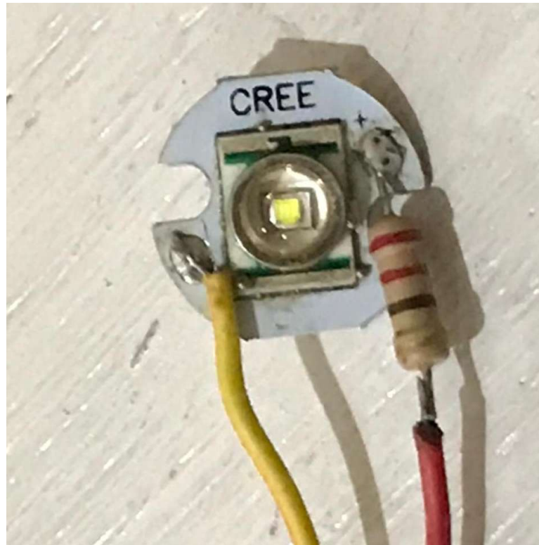
Figure 4.2: LED source along with resistor connected to limit the current flow
