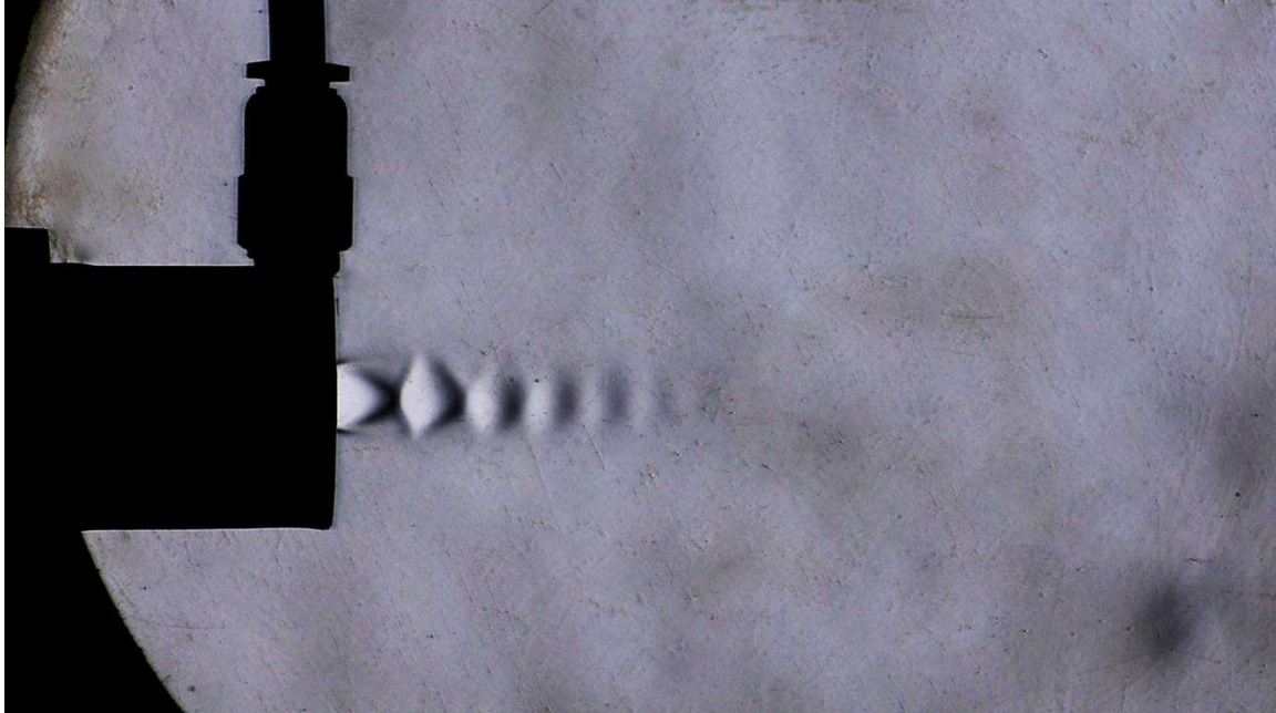
Figure 6.25: Jet deflection corresponding to NPR = 11 , SPR = 0.7 and when the secondary inlet located at (a) 25 %, (b) 50 % and (c) 75 % of the divergent section length
