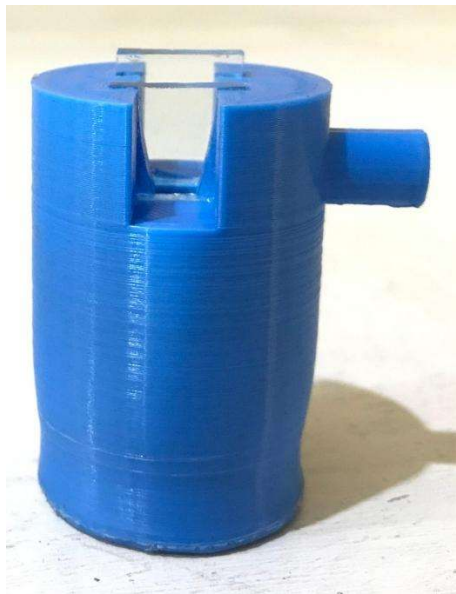
Figure 6.16: 3 D printed nozzles with transparent divergent section with secondary inlet located at 25 %
