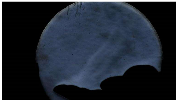
Figure 4.7: Schlieren image of hot air rising from hand
