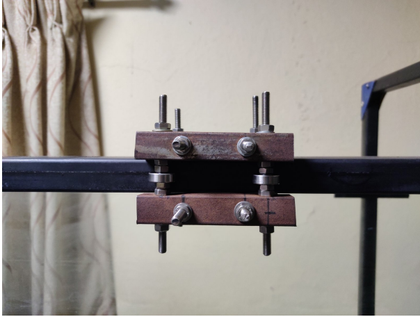
(a) Gantry roller side view
