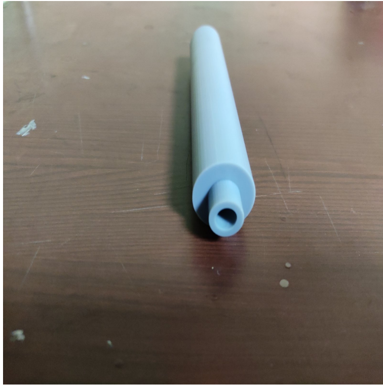
Figure 3.18: Resin Printed Circular Cylinder
