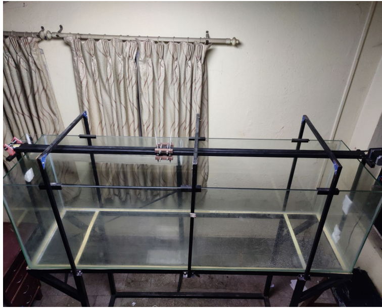
Figure 3.7: Gantry system attached to the tank setup
