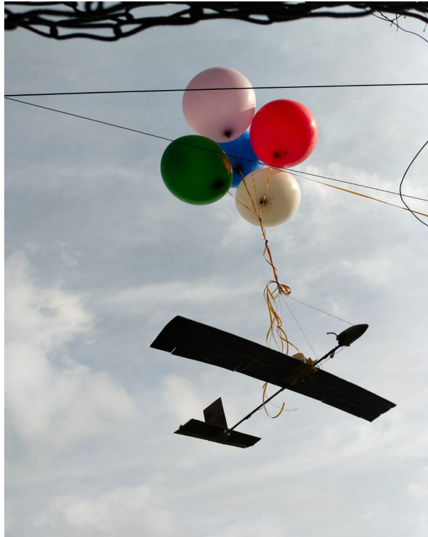
Figure 4.14: Glider prototype developed and integrate with ballon
