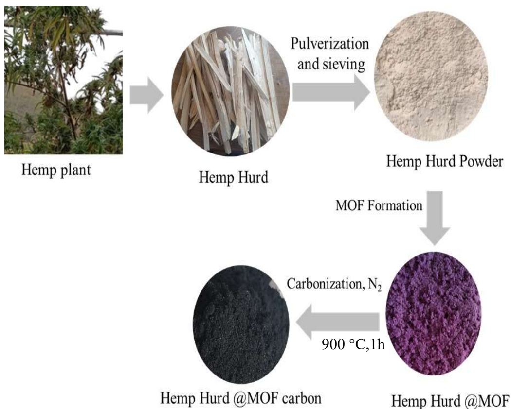
Fig. 9. Schematic Diagram of Preparation of Hemp hurd MOF Carbon
