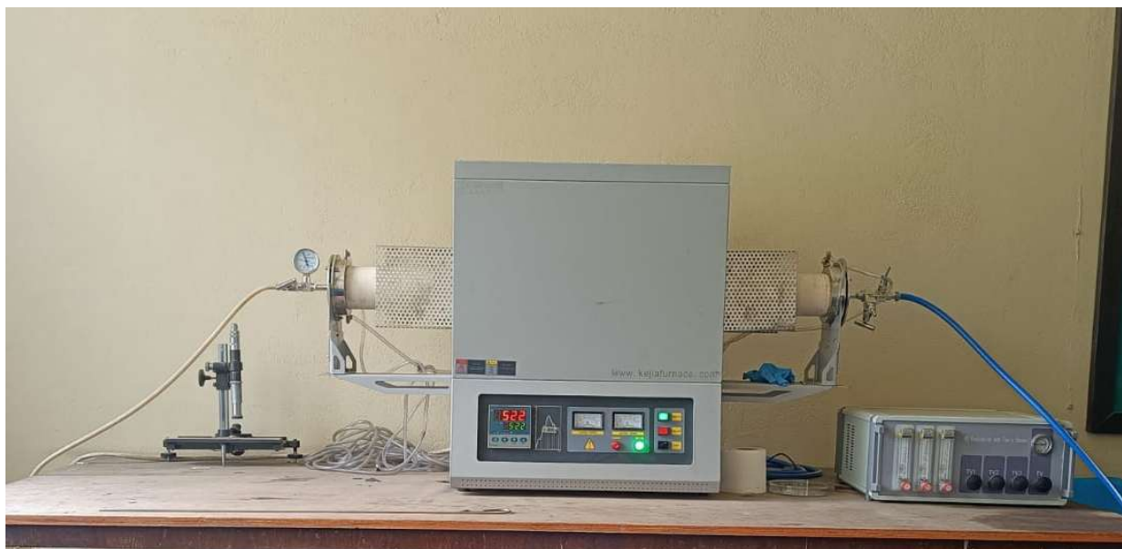
Fig. 6. Tube Furnace for Carbonization of samples
