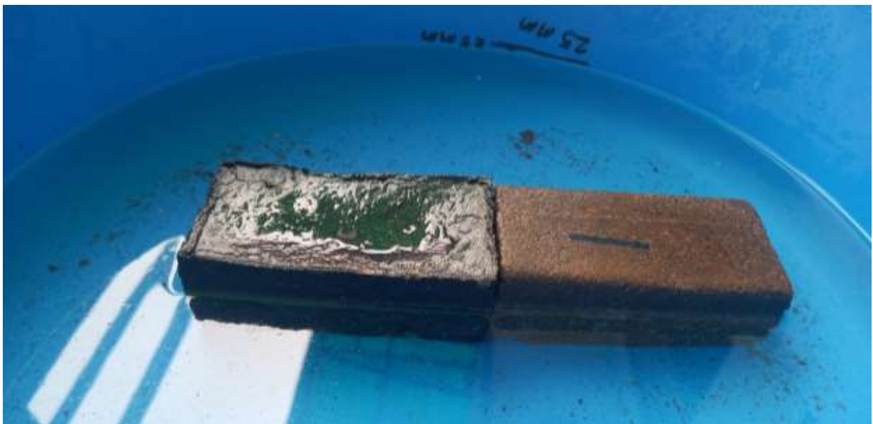
Figure 13: Efflorescence test of composite sample
