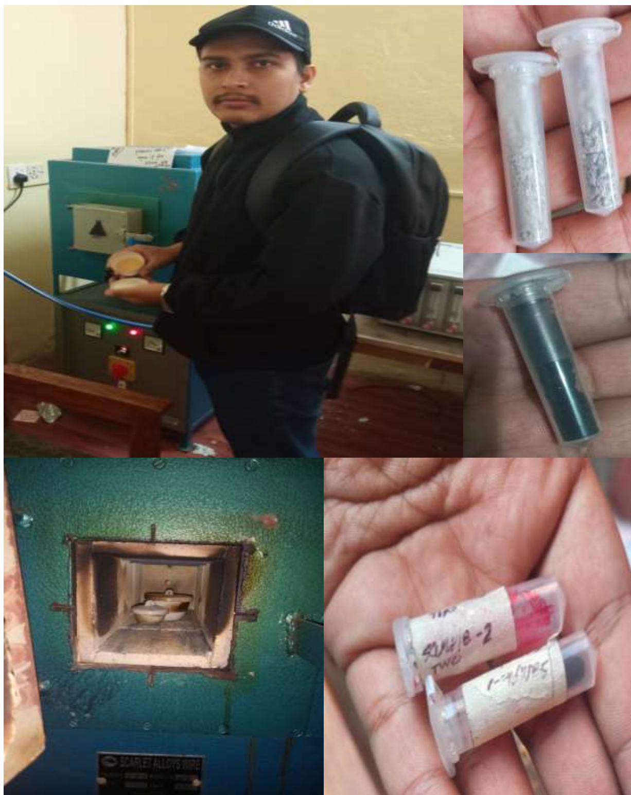
Figure 23: Making biochar and ash inside muffle furnace
