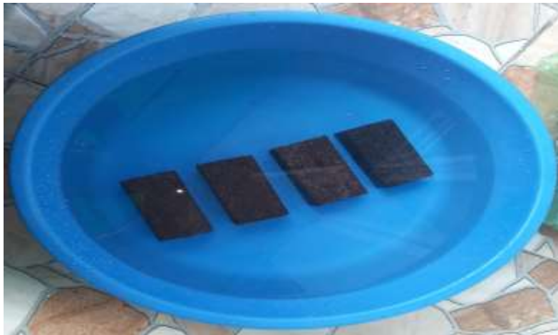
Figure 12: Composite samples placed inside water tank for water absorption test
