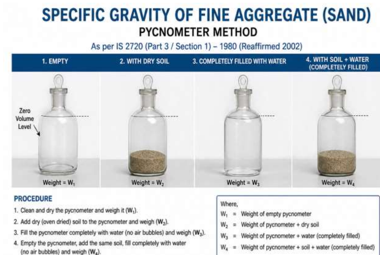
Figure 7: Testing procedure of specific gravity of sand using pycnometer
