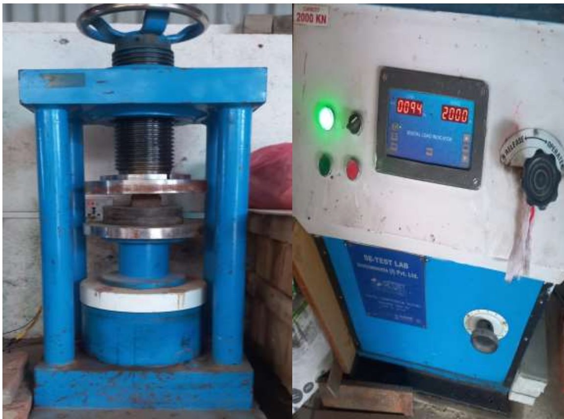
Figure 11: Compression test and data of the composite sample
