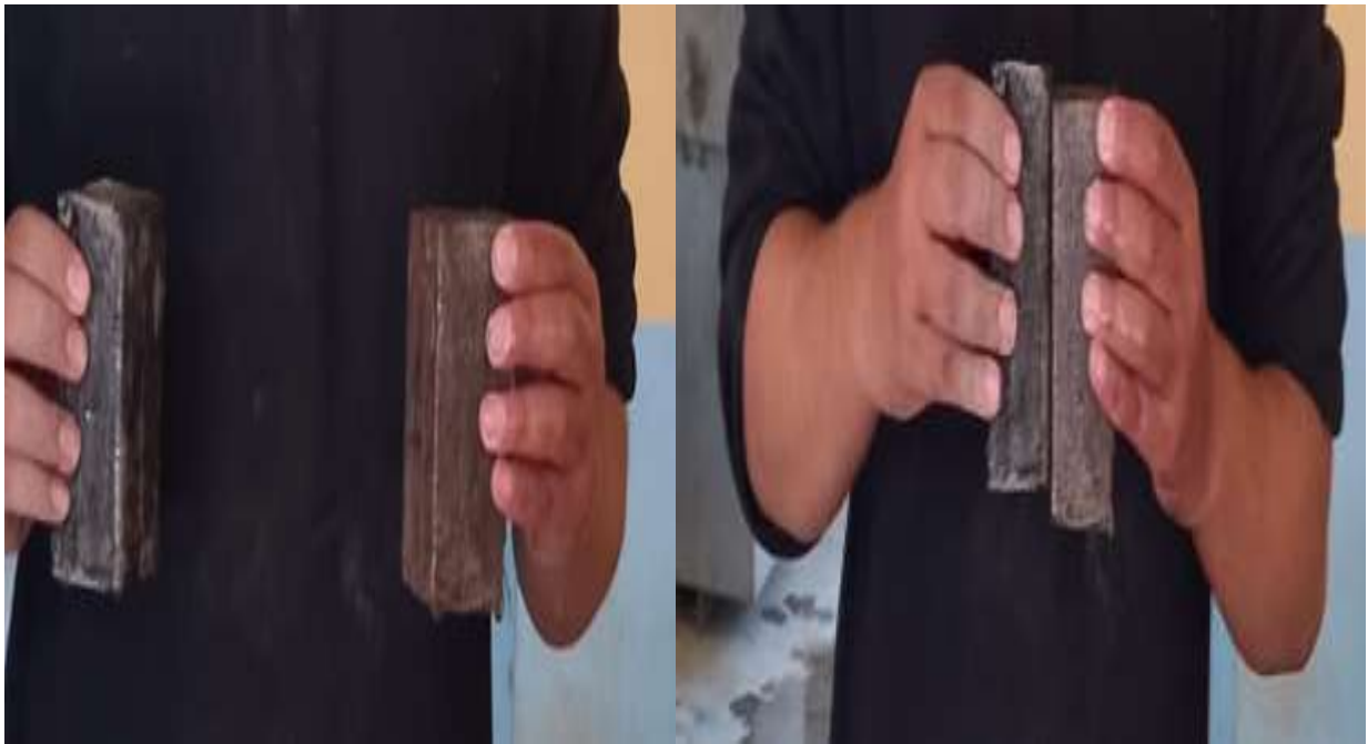
Figure 16: Ringing test of composite samples
