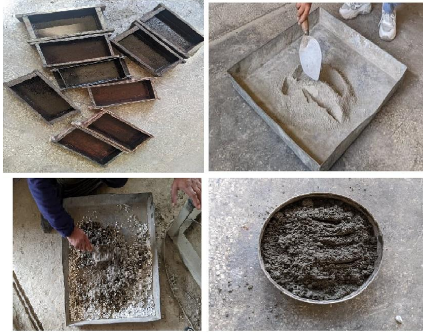
Figure 3 Wood moulds (240 mm x 115mm x 57mm) and batched materials
