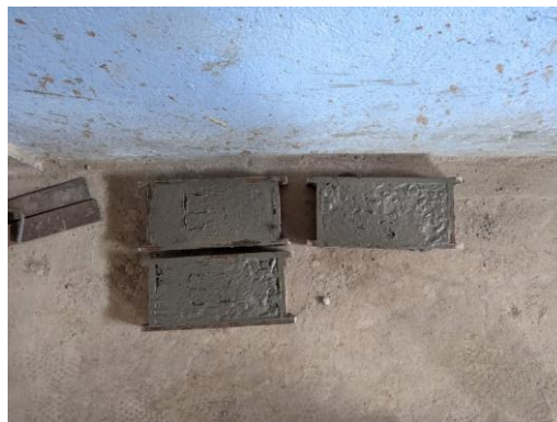
Figure 4 concrete mix in the mould
