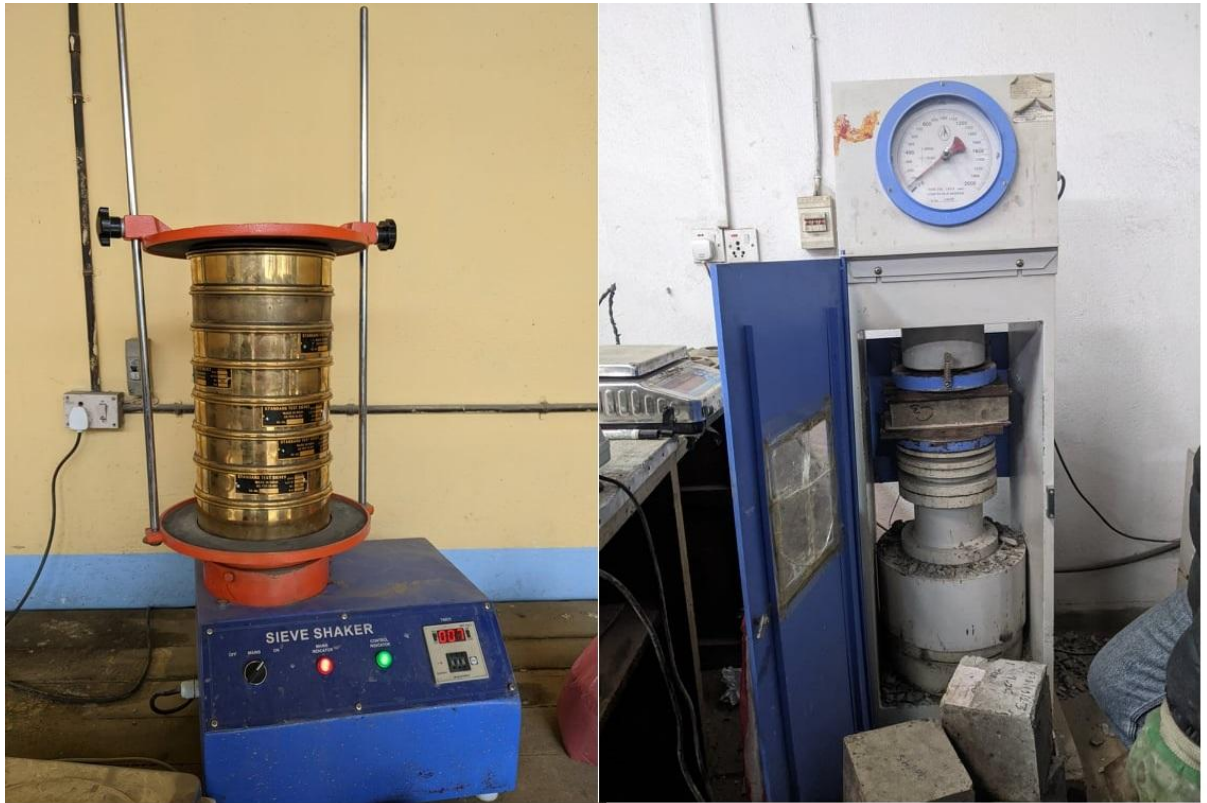
Figure 2 Sieve sets as per IS standard, sieve shaking machine and compressive strength testing machine
