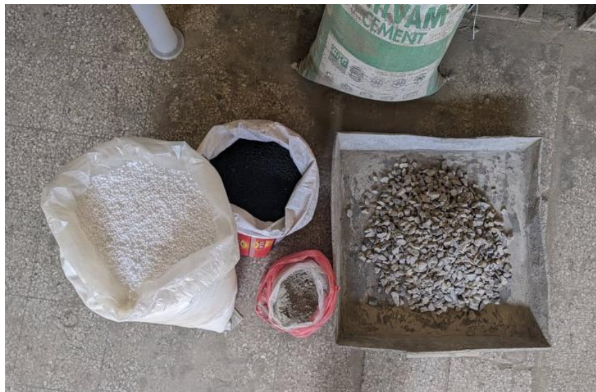
Figure 1 Cement, Coarse aggregate, EPS, Sand, Crumb Rubber
