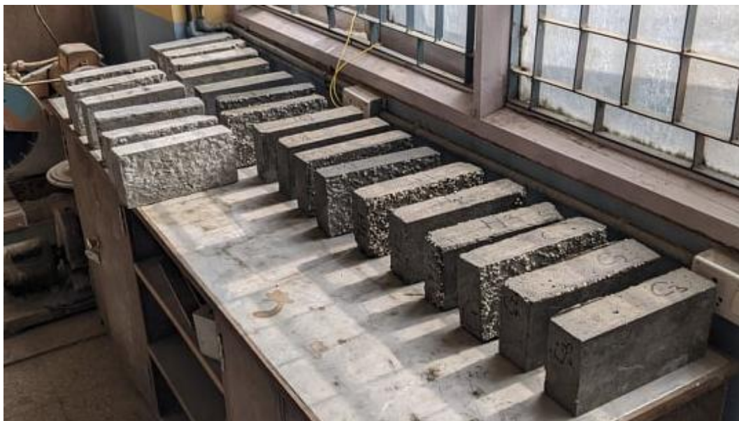
Figure 5 Prepared and cured dry 24 sample (A, B, , D, E,F, G, H) ready for compressive strength test
