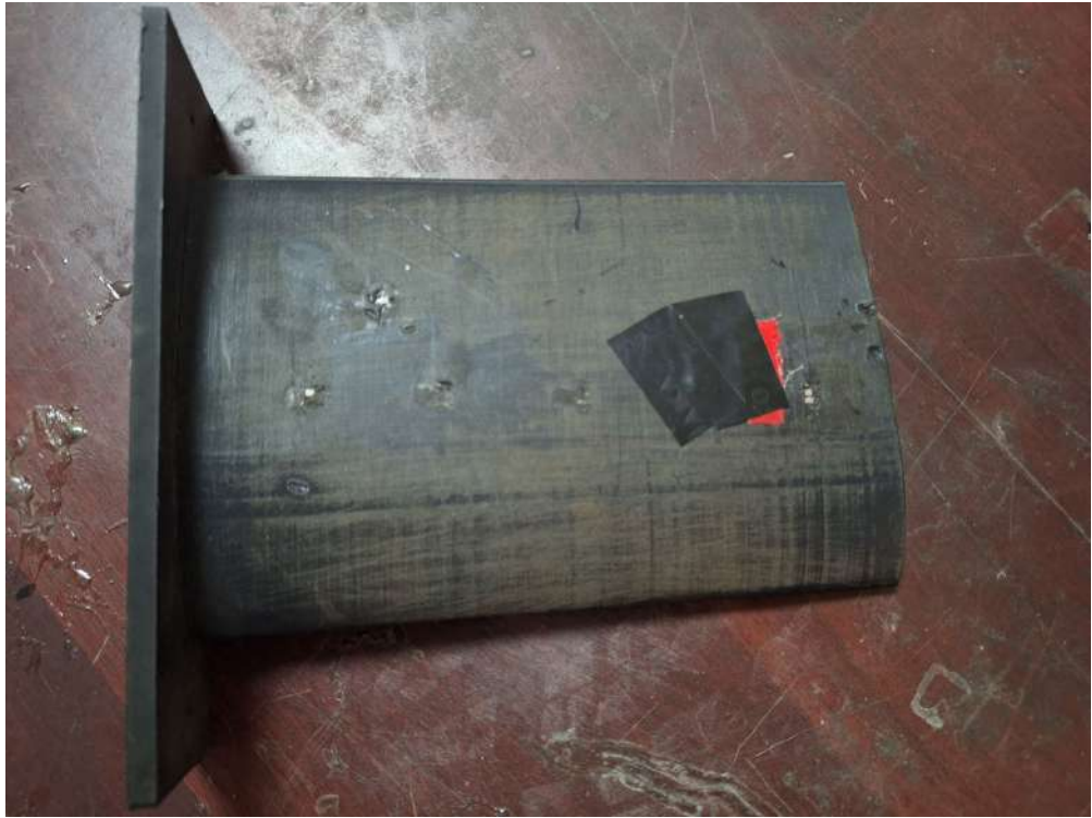
Figure B.2: 3d printed wing model
