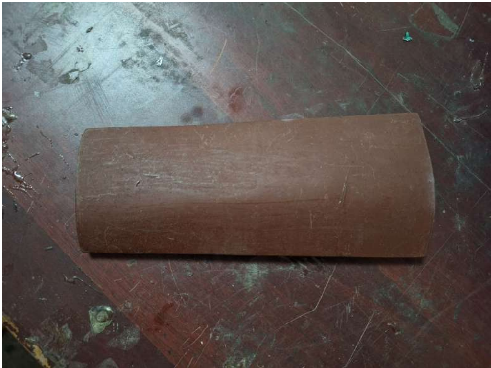
Figure B.3: Fiber fabricated wing model
