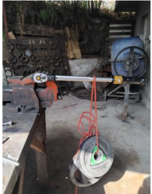
Figure VI (b): Torque wrench calibration setup with known weights
