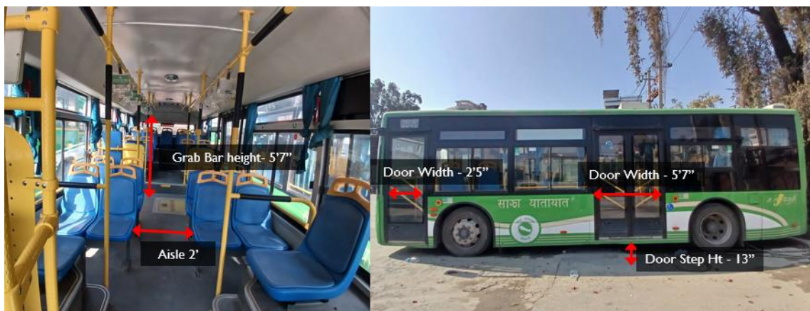
Figure 0.9 Sajha Electric Bus Design Dimension
