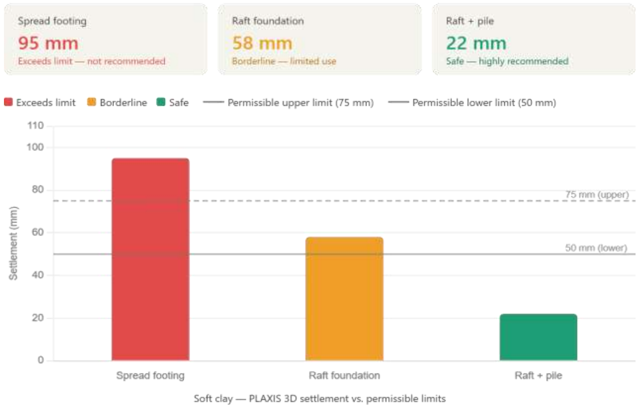
Figure 5.10 : Settlement vs permissible limits soft clay
