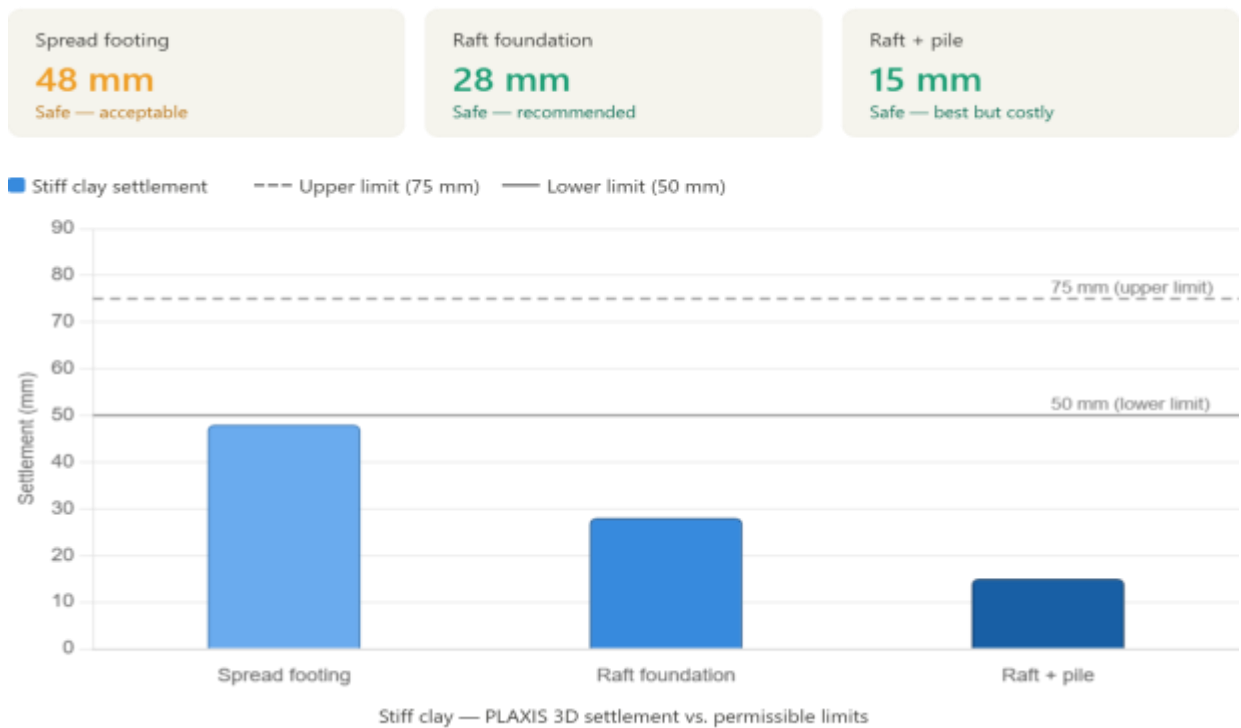
Figure 5.11 : Settlement vs permissible limit stiff clay
