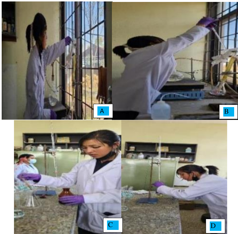
Fig: (A-B) Pipetting digested material into distillation flask (C) Pouring boric acid into conical flask (D) Titration of mixture of boric acid and ammonia with hydrochloric acid
