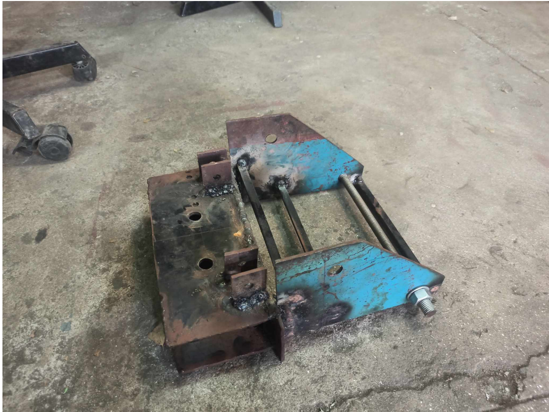
Figure 4.7: Fabricated Elastic Band Holding System
