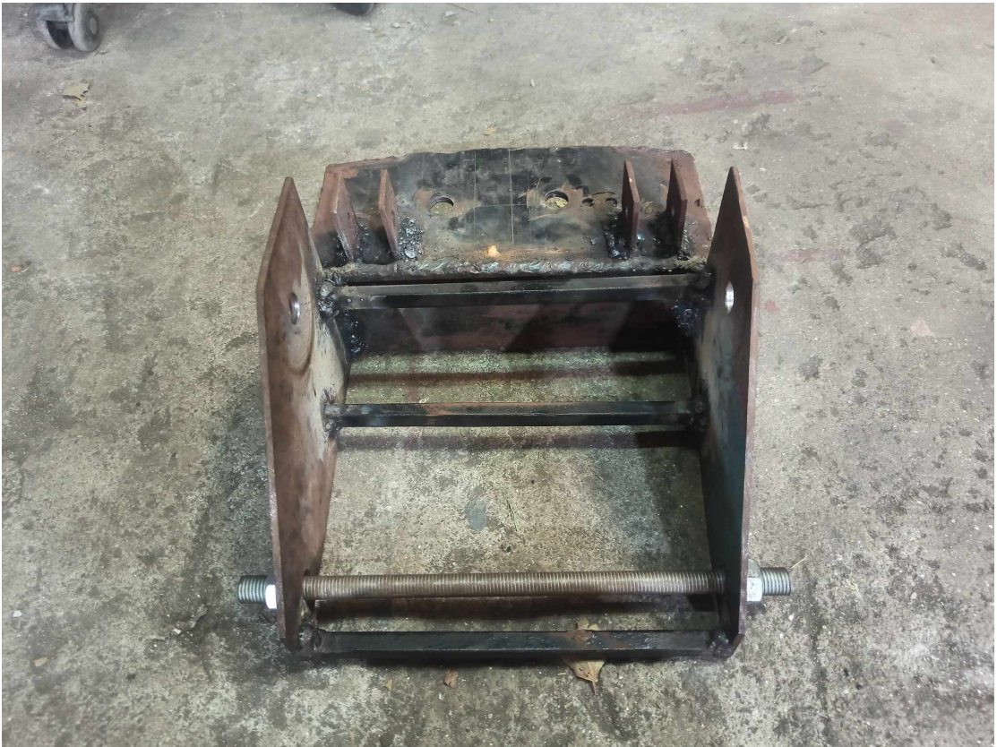
Figure B.8: Elastic Band holding system
