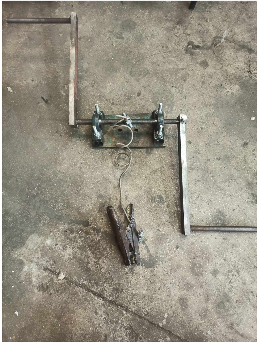
Figure 4.3: Fabricated Winch Assembly
