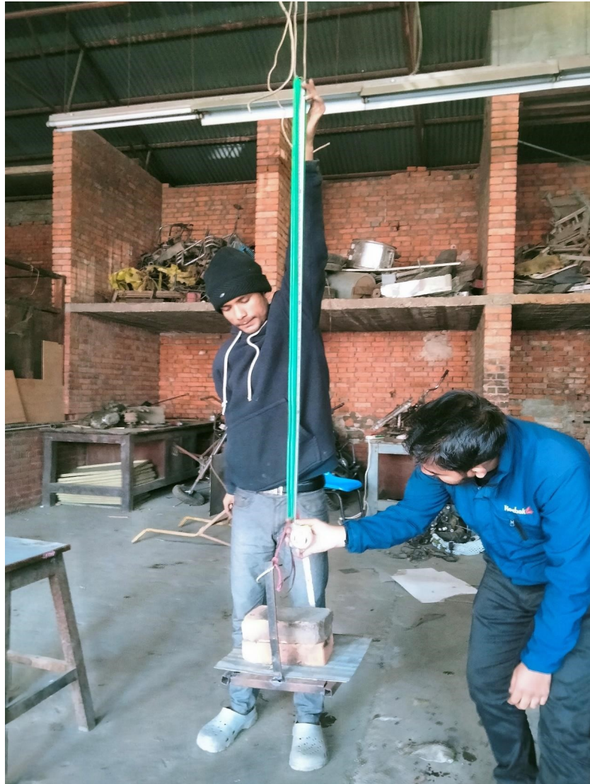
Figure 4.8: Calculation of Stiffness of Elastic band
