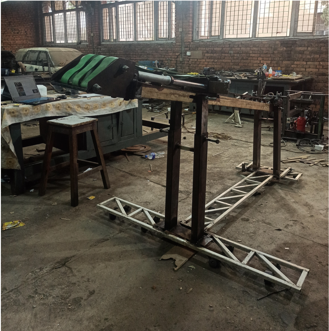
Figure B.1: Fabricated UAV Launcher
