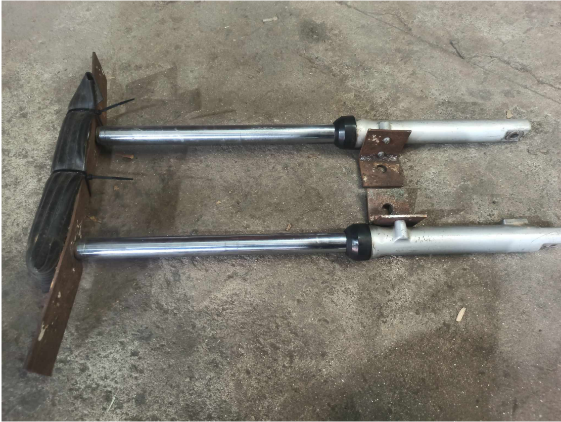
Figure 4.6: Fabricated Damping Mechanism
