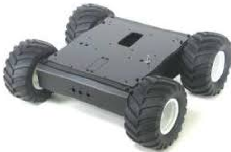
Figure 2.3: Skid-Steer Drive Robot[4]
