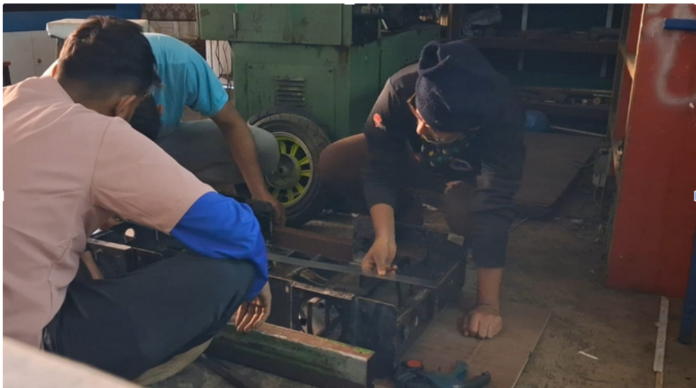
Figure 2: Measuring and Verifying the Dimensions of the Setup Before Welding
