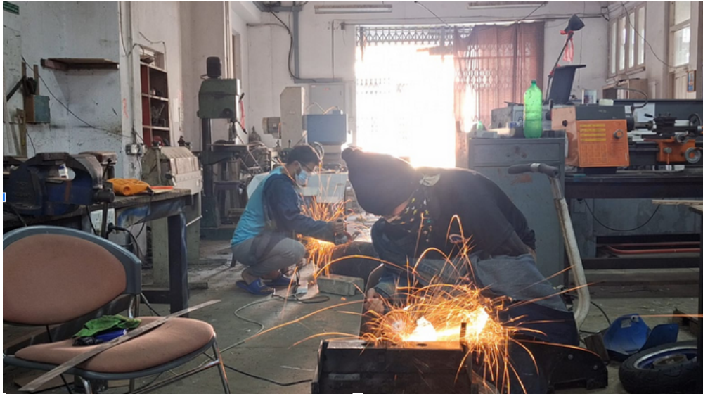
Figure 1: Grinding the Hoverboard's Chassis for Proper Alignment During Assembly
