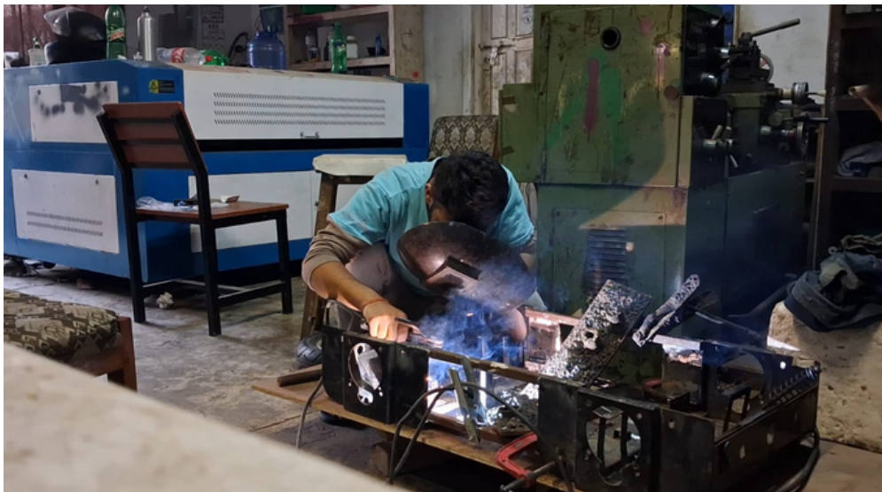
Figure 4: Chassis Fabrication in Progress through Welding
