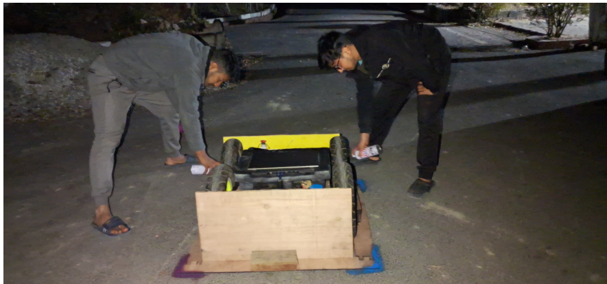
Figure 4.15: Marking Position of Robot with Jig
