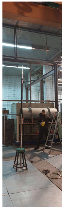
Figure 2. 16: Air termination under test
