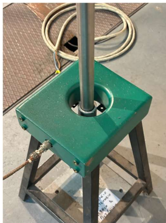
Figure 2. 18: Current measurement through a current transformer
