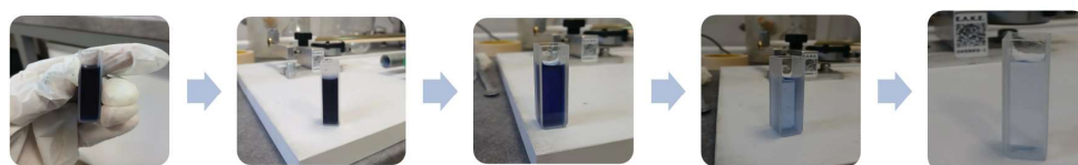
Figure 4.9: Photocatalytic degradation of methylene blue under UV ( A_0 = 1.315 , \lambda = 664\text{ nm} )
