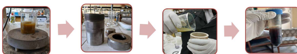
Figure 3.2: Diagrammatic representation of the Hydrothermal process
