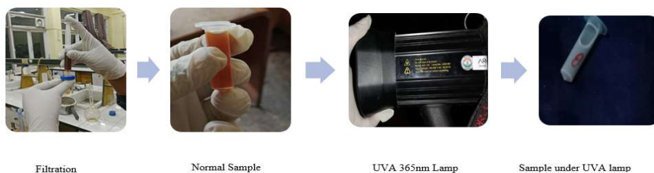
Figure 4.2: Testing of Undiluted sample in the UVA 365nm lamp
