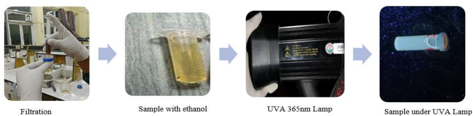
Figure 4.3: Testing of Ethanol diluted sample in the UVA 365nm lamp
