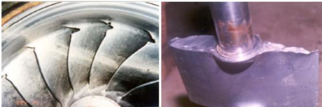
Figure 2. 11 Wear caused by sediment erosion on the Francis turbine's runners and guiding vane in Jhimruk (Thapa, 2015)
