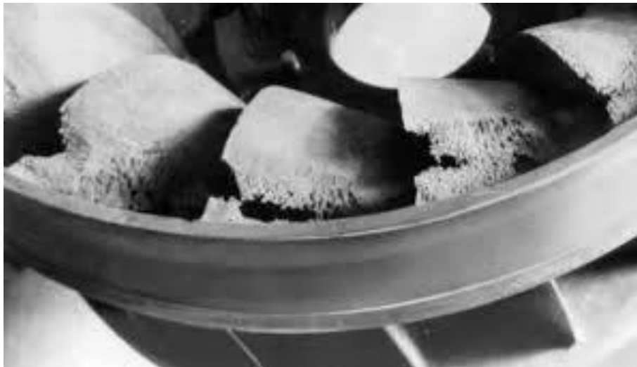
Figure 1. 1 Cavitation damage on the blades at the discharge from a Francis turbine (Brennen, 2011)
