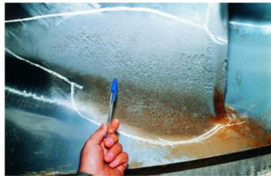
Figure 2. 3 Cavitation damage on runner blade surface (Subramanya, 2013)
