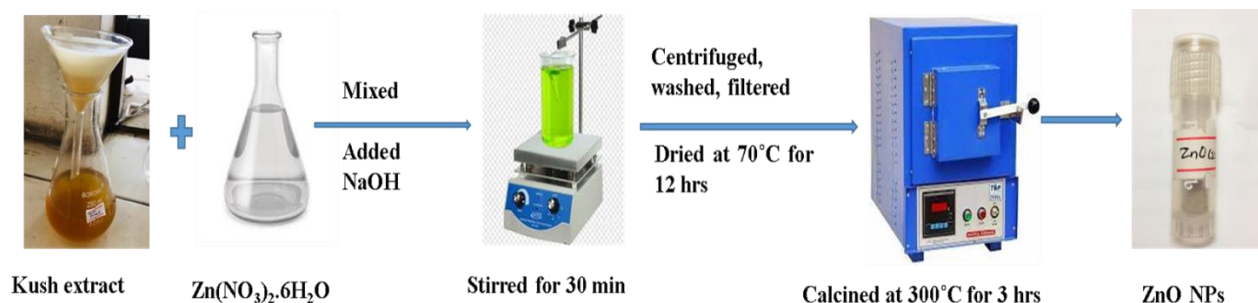
Figure 3.3: Schematic representations for the green synthesis of ZnO NPs.
