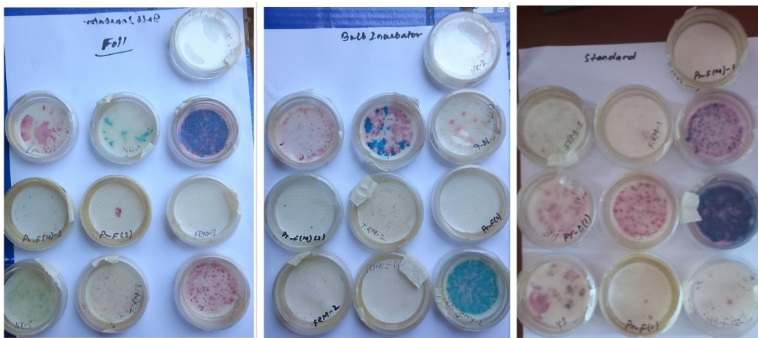
Photo 11: Results of three sets of water samples tested in foil, bulb, and standard incubator
