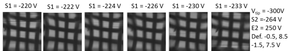
Fig. 4.13 S1 variation for the best surface current electron micrograph for fixed E2 and S2 voltages.
